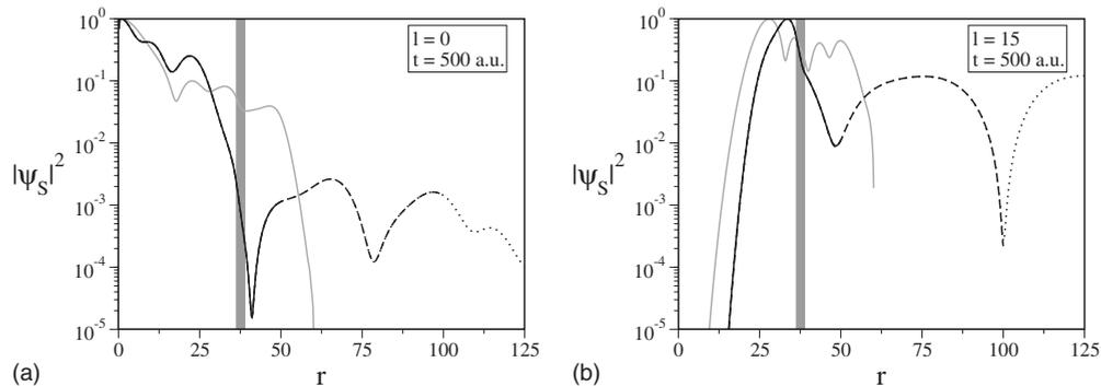
FIG. 4. Comparison of the reference solution to a boundary at  $R=2000$  (dotted) to solutions with radiation boundary conditions at  $R=50$  (solid) and  $R=100$  (dashed) and to the solution with absorbing boundary conditions in a region between  $R=50$  and  $R=60$  (gray) after  $10^4$  time steps. Shaded bar indicates the position of the potential well. Simulation parameters:  $E_0=0.5$ ,  $r_0=25$ ,  $R_1=36.25$ ,  $R_2=38.75$ ,  $V_0=0.1$ ,  $\Delta t=0.05$ ,  $\Delta r=0.1$ .
