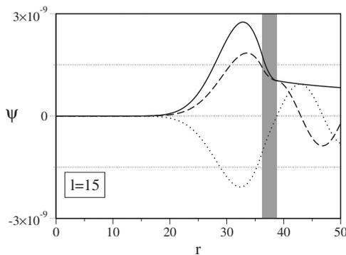
FIG. 6. A snapshot of the wave function for  $l=15$ ,  $E_0=0.5$ ,  $R_1=36.25$ ,  $R_2=38.75$ ,  $V_0=0.1$ ,  $\Delta t=0.05$ , and  $\Delta r=0.1$  at time  $t \approx 2500$ . Shaded bar shows the position of the finite potential. Dashed: real part, dotted: imaginary part, solid line: modulus.
