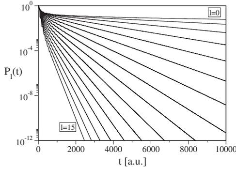
FIG. 8. Time history of the probability  $P$  to find the particle in the computational volume. Simulation parameters:  $E_0=0.5$ ,  $R_1=36.25$ ,  $R_2=38.75$ ,  $V_0=0.1$ ,  $\Delta t=0.05$ ,  $\Delta r=0.1$ . The decay rate rises with the parameter  $l$ .
