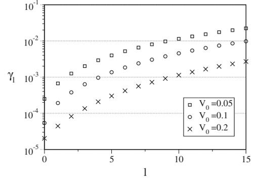
FIG. 9. Static decay rate  $\gamma_l$  as a function of the quantum number  $l$  for various heights  $V_0$  of the finite barrier. Simulation parameters:  $E_0=0.5$ ,  $R_1=36.25$ ,  $R_2=38.75$ ,  $\Delta t=0.05$ ,  $\Delta r=0.1$ .
